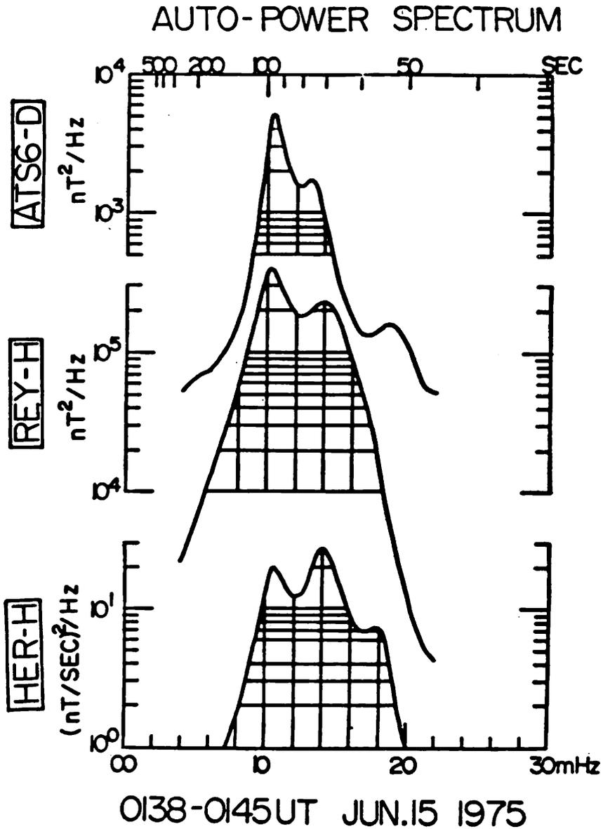
Fig. 3. The maximum entropy method of spectral analysis was applied to the  $Pi$  wave trains illustrated in Fig. 2 for the interval of 0138-0145 UT. The common spectral component can be seen around 11 mHz both in the magnetosphere and on the ground.
