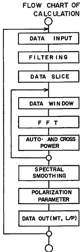
Fig. 21. Flow chart showing calculation procedure of polarization parameters.
