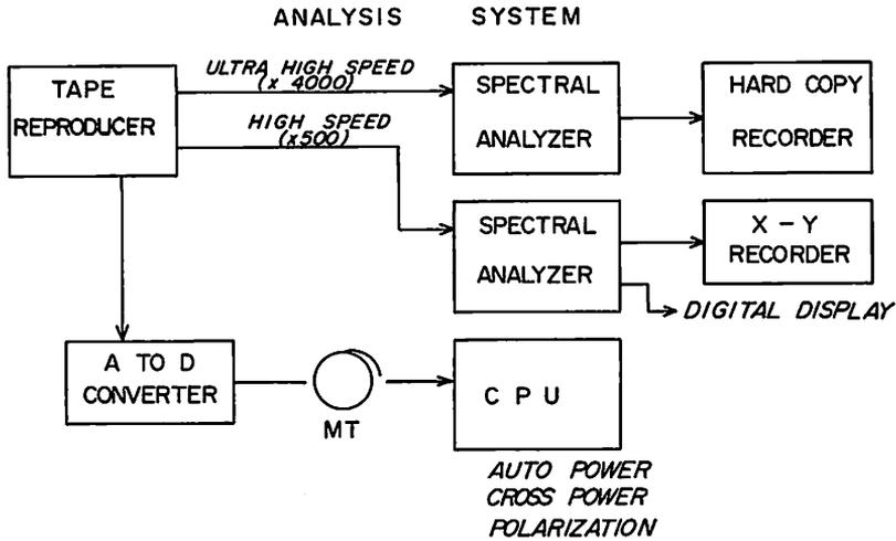
Fig. 4. Block diagram of pulsation analyzing system installed at the Kakioka Magnetic Observatory. But analysis of the polarization characteristics was carried out by a computer system of the National Institute of Polar Research.
