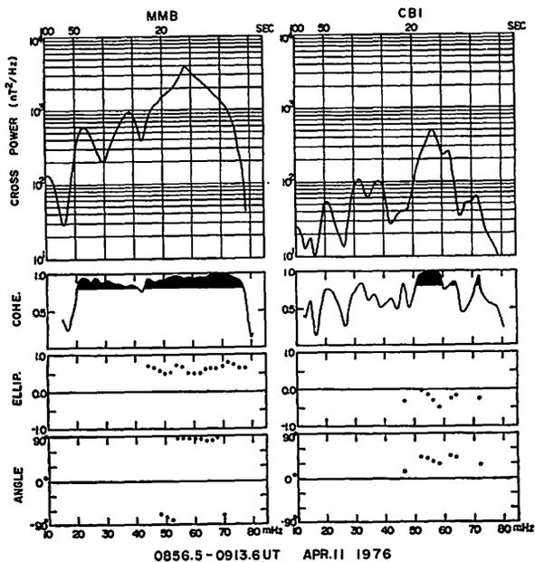
Fig. 29. Cross-power spectrum, coherency, ellipticity and direction angle of the major axis of the pulsation pc-3 shown in Fig. 28.
