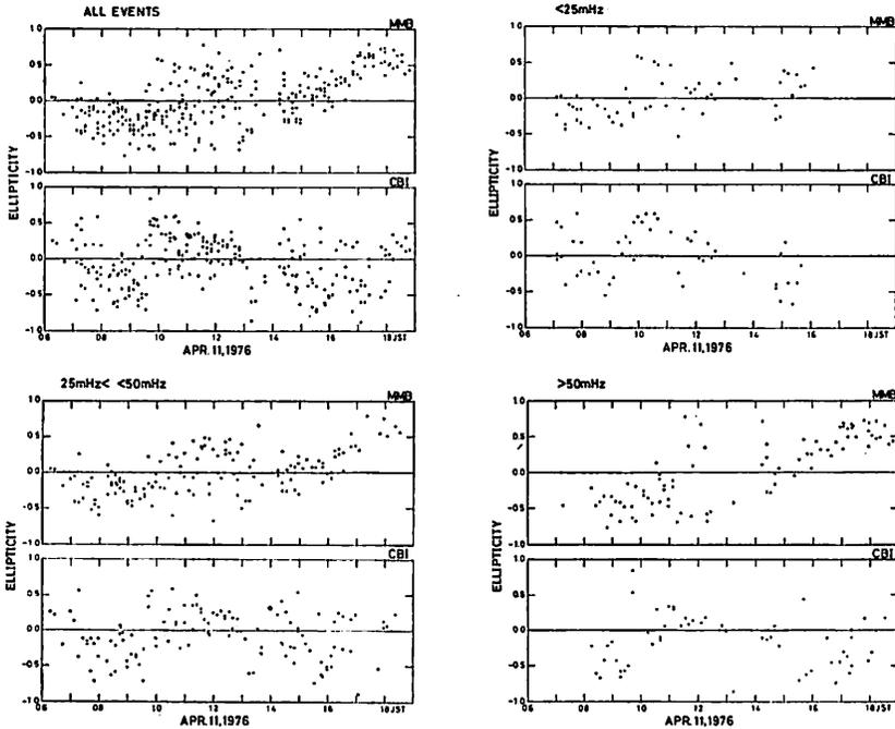
Fig. 30. Diurnal variations of ellipticity in full, less than 20 sec, 20-40 sec and more than 40 sec ranges, respectively. The upper and lower diagrams correspond to the variations at Memambetsu and Chichijima.
