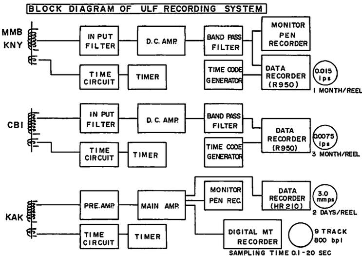
Fig. 1. Block diagram of pulsation observing systems at four observatories, Memambetsu, Kanoya, Chichijima and Kakioka.
