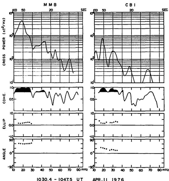
Fig. 25. An example of polarization analysis for pi-2 observed at Memambetsu and Chichijima. The top, second, third and bottom diagrams show cross-power spectrum, coherency, ellipticity and direction angle of the major axis, respectively.
