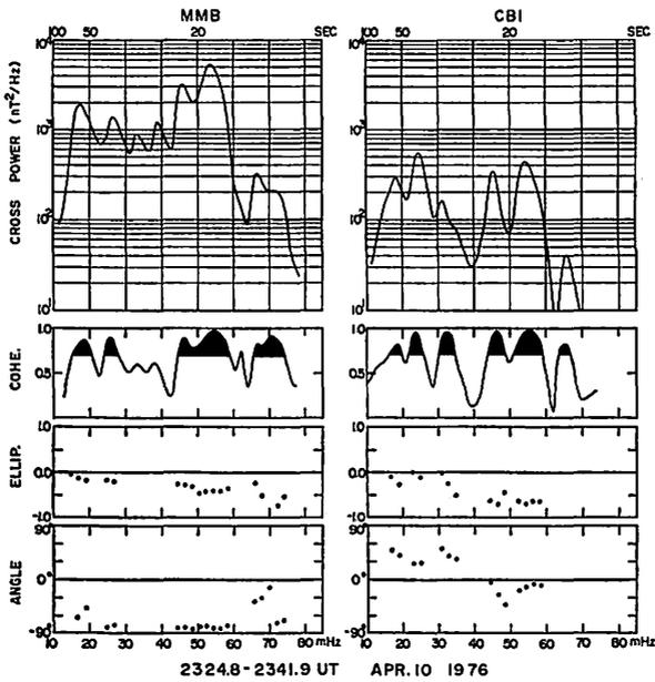
Fig. 27. Cross-power spectrum, coherency, ellipticity and direction angle of the major axis of the pulsation pc-3 shown in Fig. 26.
