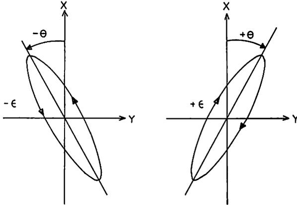
Fig. 22. Definition of signs of polarization characteristics (ellipticity and direction angle of the major axis) in our calculation program.
