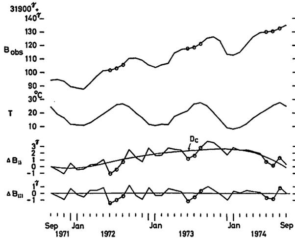
Fig. 4. Analysis of base-line values for Kanoya's No. 2 Z-variometer (I).
