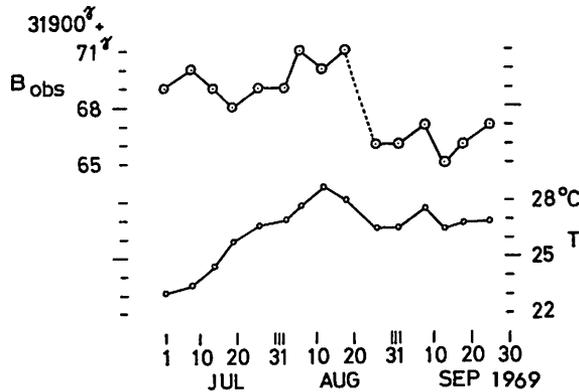
Fig. 2. Weekly observed base-line values and temperatures of Kanoya's No. 1 Z-variometer in July, August and September of 1969.
