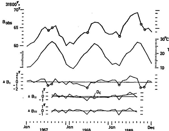
Fig. 1. Analysis of base-line values for Kanoya's No. 1 Z-variometer. For  $D_c$ , see Eq. (7).
