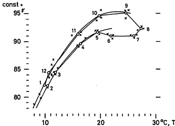
Fig. 6. Temperature-dependence of base-line values of Kanoya's No. 2 Z-variometer with the drift,  $1.133t + Dc$ , subtracted.
