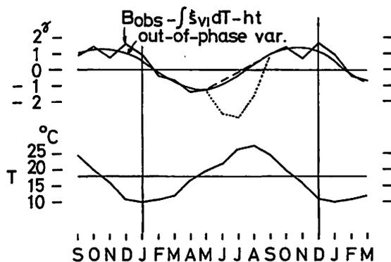
Fig. 10. Mean annual variation of the residual of base-line values shown at the top of Fig. 9 (upper) and temperatures (lower). A smooth curve in the upper part is the out-of-phase variation with respect to the annual term of temperature change when  $k=0.0819 \gamma/\text{month}/^\circ\text{C}$ .
