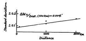
Fig. 26 The relrtion between the standard deviations of the 5-day-mean values from their yearly mean values and the distance of the observatories in 1964 (declination).
