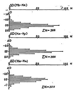
Fig. 19 The distributions of the deviations of the differences of the daily mean values from their yearly mean values betwen the observatories in 1964 (declination).
