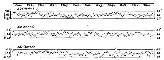
Fig. 17 The deviations of tht differences of the daily mean values from their yearly mean values between the observatories in 1964 (declinations).
