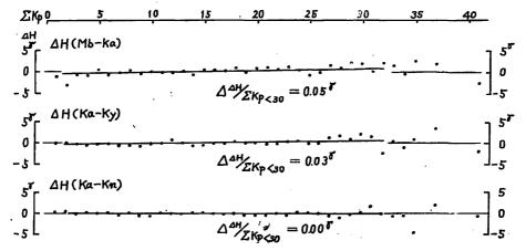
Fig. 5 The relations between the deviations of the differences of the daily mean values from their yearly mean values and  $\sum K_{\rho}$  in 1964 (horizontal intensities).
