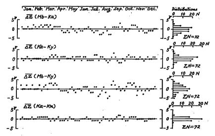
Fig. 23 The deviations of the differences of the 5-day-mean values from their yearly mean values between the observatories in 1964 (vertical intensity).
