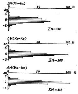
Fig. 6 The distributions of the deviations of the differences of the daily mean values from their yearly mean values between the observatories in 1964 (horizontal intensity).
