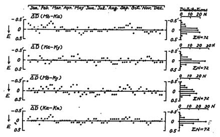
Fig. 25 The deviations of the differences of the 5-day-mean values from their yearly mean values between the observatories in 1964 (declination).
