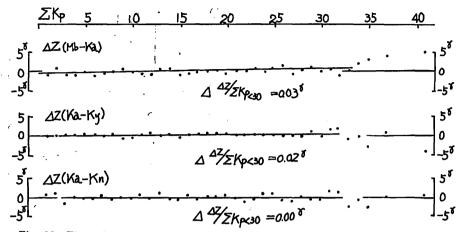
Fig. 12 The relations between the deviations of the differences of the daily mean values from their yearly mean values and  $\sum K_{\rho}$  in 1964 (vertical intensity).
