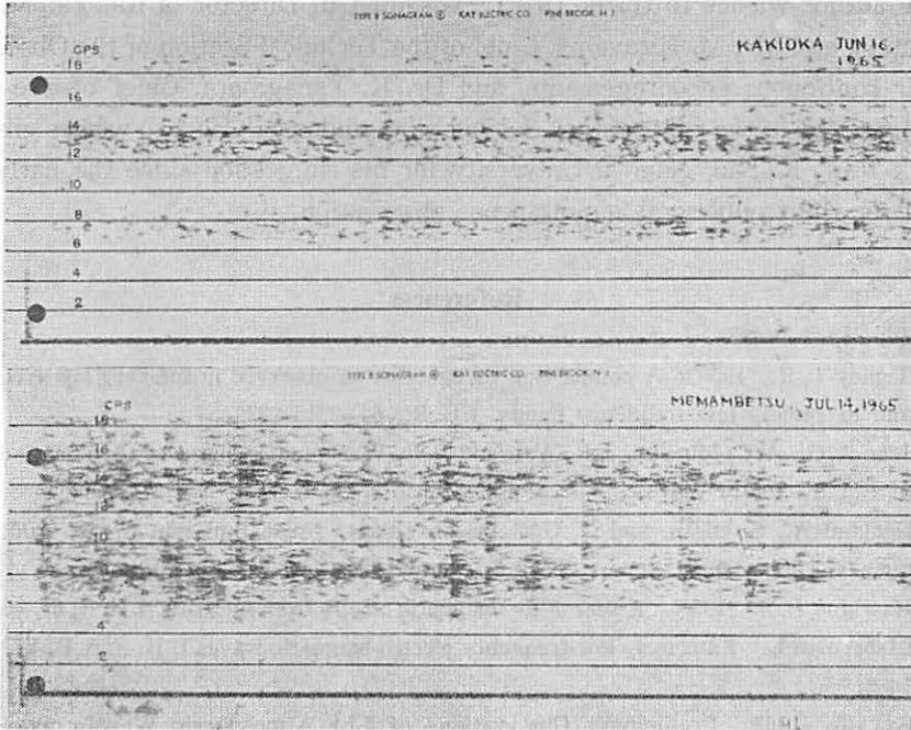
Fig. 16 An example of sonagram of received signal at Kakioka and Memambetsu.
