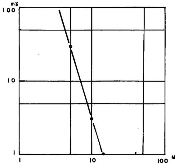
Fig. 3 The rate of decrease of the pulse coming from the artificial noise source.
