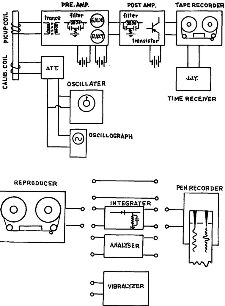
Fig. 7 The overall construction of the observational equipment with the loop antenna.
