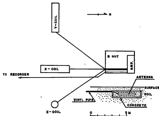
Fig. 4 The arrangement of the loop antenna.
