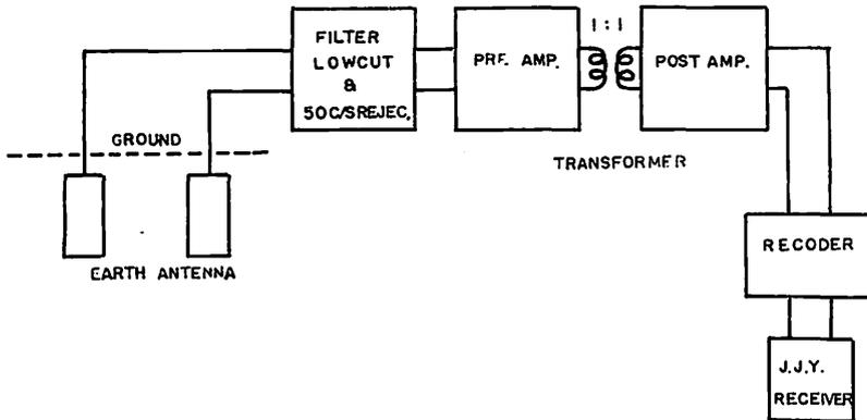
Fig. 10 The overall construction of the equipment with the earth-antenna.
