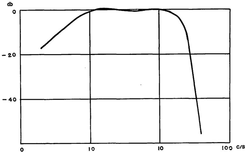
Fig. 11 The overall frequency response of the equipment with the earth-antenna.
