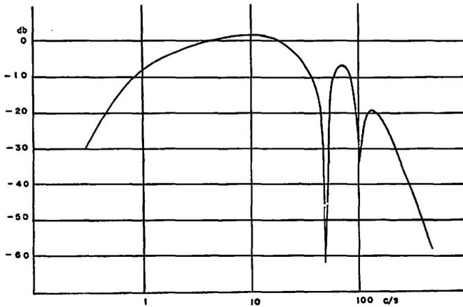
Fig. 6 The frequency response of the amplifier.
