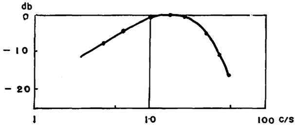
Fig. 8 The overall frequency response of the equipment with the loop antenna.
