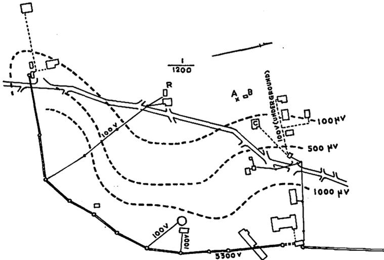
Fig. 2 The plan of the premises of the Kakioka Magnetic Observatory and the distribution of 50 cps noise.
