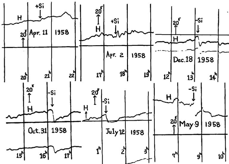
Fig. 2. Reproductions of normal-run magnetograms of Kakioka recording si's whose equivalent current system are obtained.
