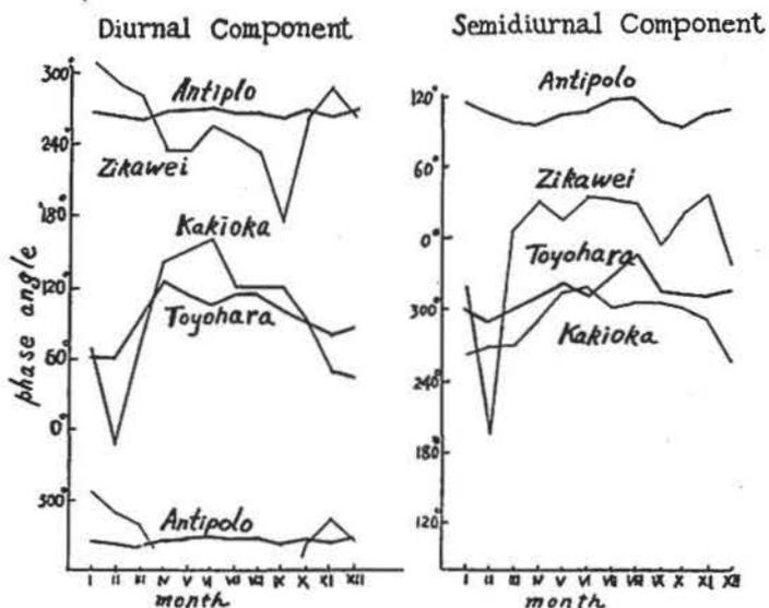
Fig. 3b. Annual variation of phases of diurnal and semidiurnal components of H at four stations in the Far East.
