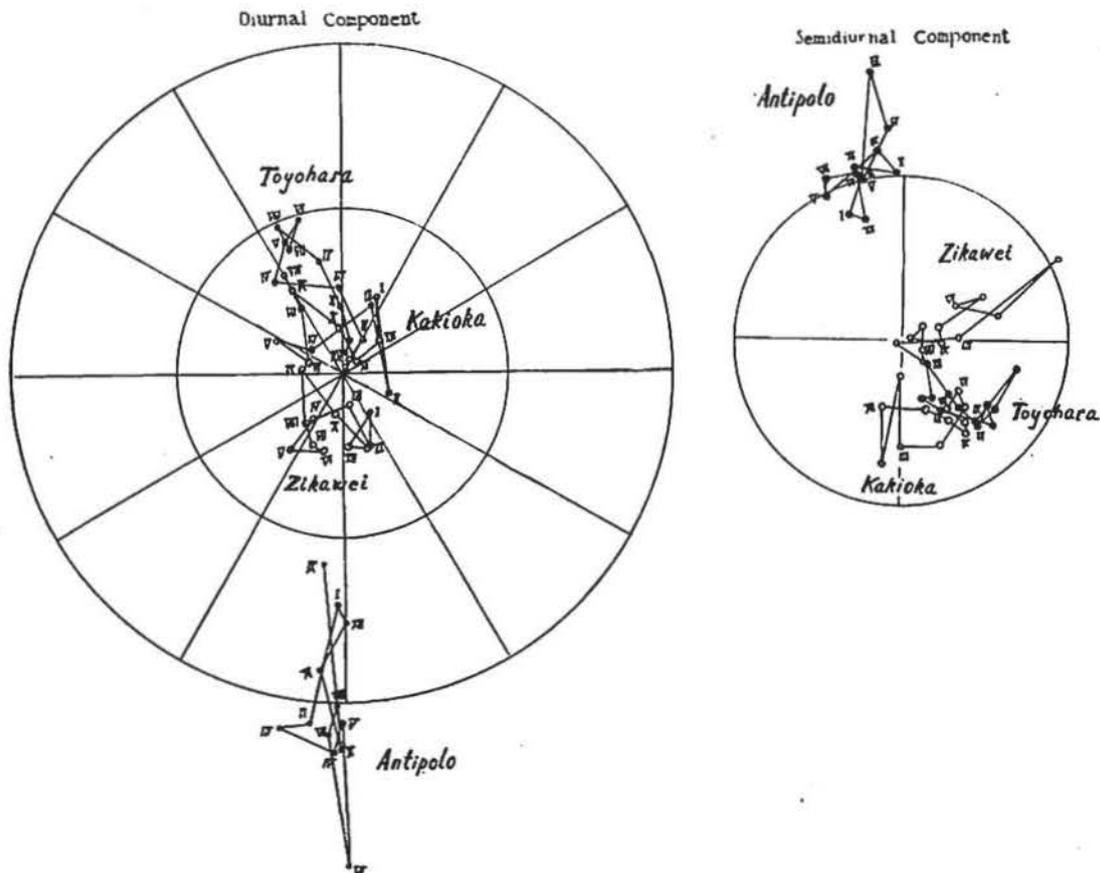
Fig. 3a. Harmonic dials for diurnal and semidiurnal components of H at four stations in the Far East.
